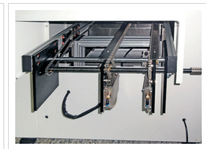
入口传动与清洗系统 Inlet drive and cleaning system
