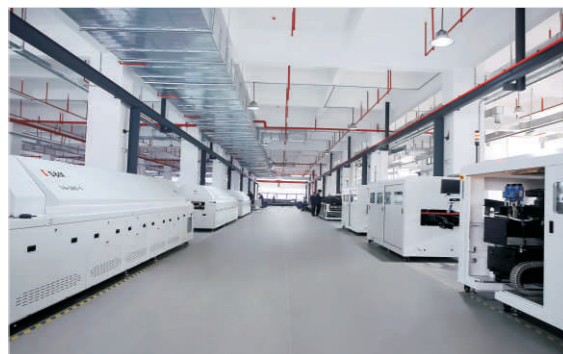
回流焊装配车间 Reflow oven assembly shop
